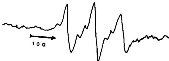
FIGURE 5 ESR spectrum of bifnox ( 10^{-2}M/l ) and TME ( 5.10^{-2}M/l ) in Brij 35 micelle medium.
